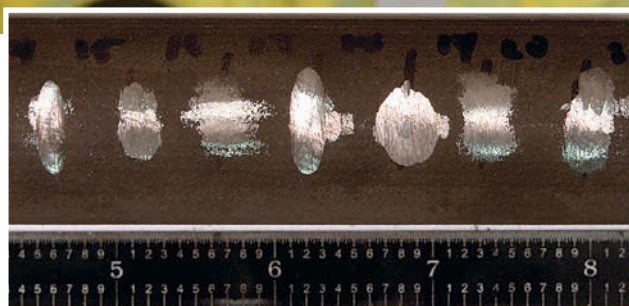
Above, Danny Nguyen, a sheet metal mechanic at Tinker AFB, Okla., repairs a panel for a KC-135 vertical stabilizer. USAF's new Rapid Sustainment Office is exploring new technologies that can cut the costs of maintenance, such as the application of cold spray technology, an additive manufacturing process that enables maintainers to restore metal parts, such as these chafed titanium tubes (left), by adding metal back where it has been worn away. Depots at Tinker, (above) and Robins AFB, Ga., are already using the process.
